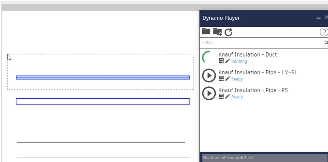
3. A Dynamo pop-up box will appear, like in the image. You have to select the wished insulation product/thickness you wish to apply to the duct/s:
