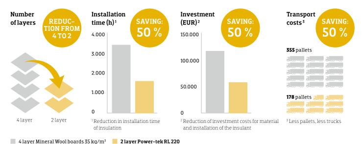
\*) Remark: Calculations are based on a real case with a technical requirement of 500 mm insulation thickness. Market prices and construction principles in different markets may have influence on the calculation, so there is a possibility of deviation.
